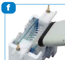
Load samples using Loading Guides and run
