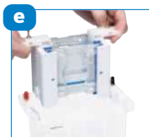
Transfer to tank and fill with buffer
