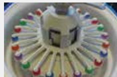
QuickPrep™ 3 Sample Holder 24 x 2 mL tubes (included with FastPrep-24™ 5G instrument) Cat. No. 116005512
