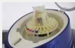
QuickPrep™ Sample Holder 24 x 2 mL tubes (included with FastPrep-24™ instrument) Cat. No. 116002512
